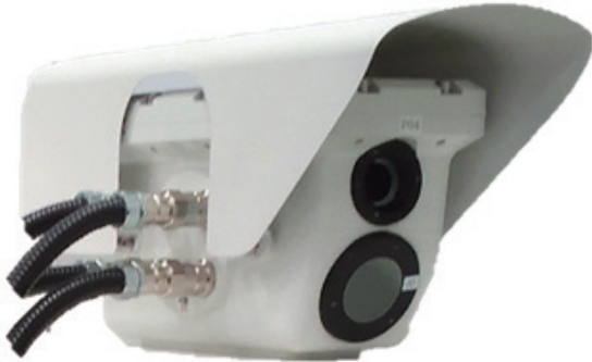
Fig. 9 The gas detection camera unit, consisting of a visible image camera and an IR camera mounted below it. The camera unit is sealed so as not to spark an explosion in the presence of gas.
